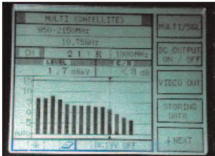
Figure 14 – 950-2150MHz – with 4-Way Splitter
